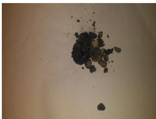
Figure 5.2. Clinkers formed during air-blown gasification
