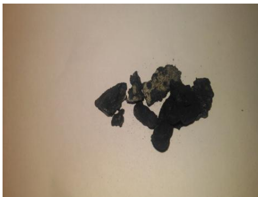
Figure 5.1. Clinkers formed during oxygen-blown gasification
