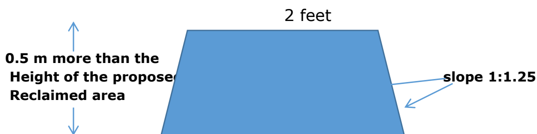
Cross- section of water body protection embankment
