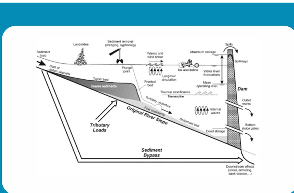
**Fig 2 Sedimentation Pattern in Reservoir (USBR, 2006)**
