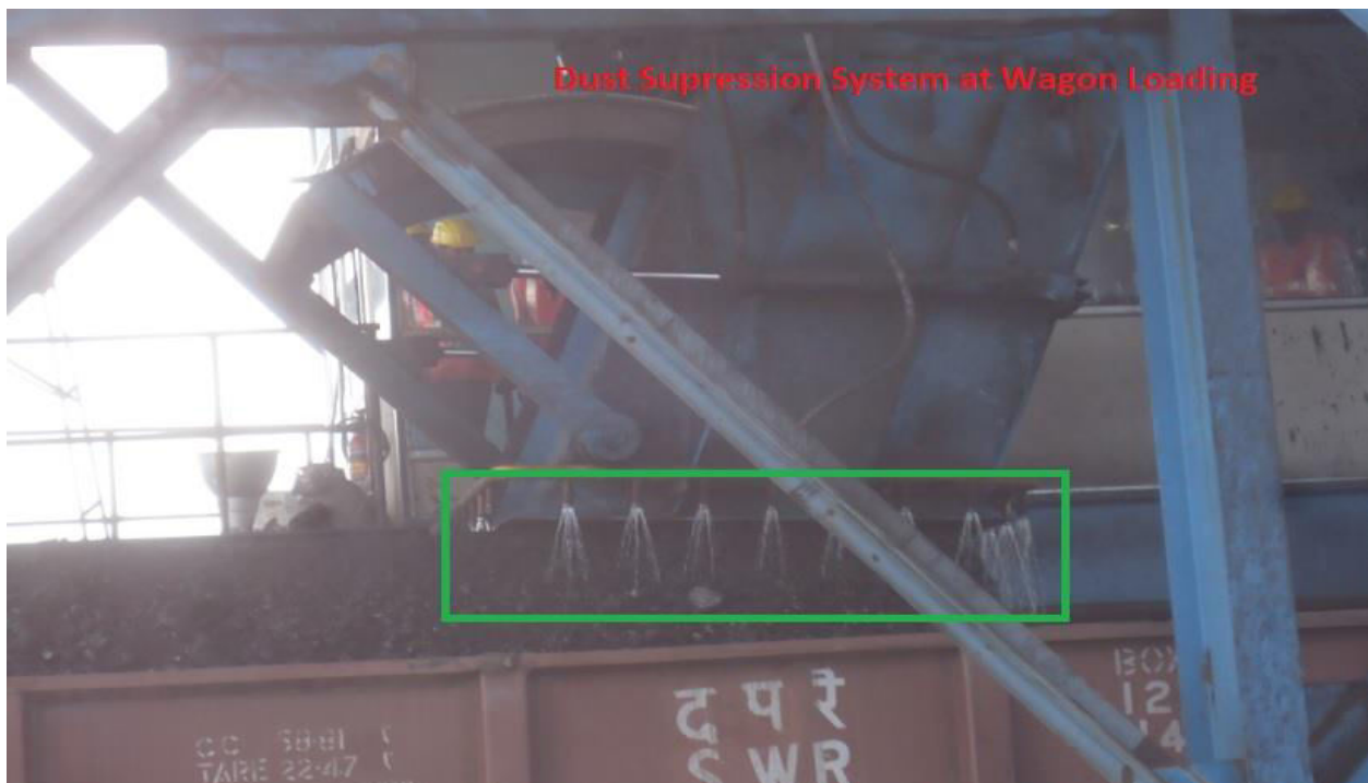
Plate-10 Coal Loading through Mechanized System to Railway wagon with Dust Suppression System
