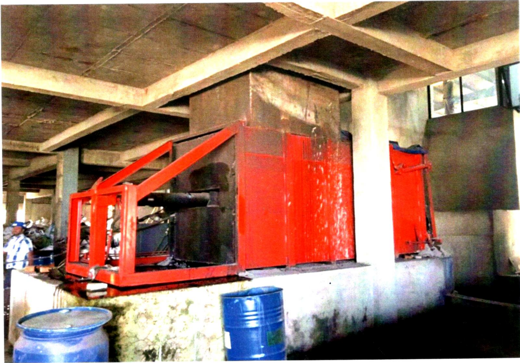
Figure 7. Proposed automation for solid waste blending - Compactor
