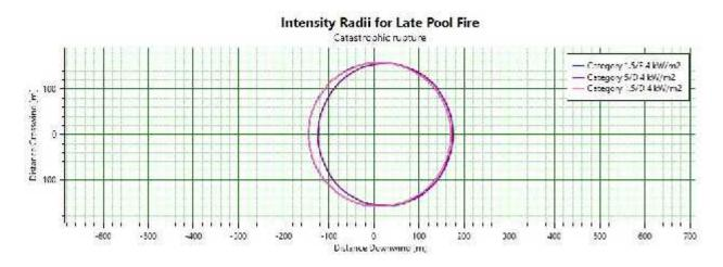
Figure 3-15 Late Pool Fire from Catastrophic rupture of Iso Propanol Storage tank
