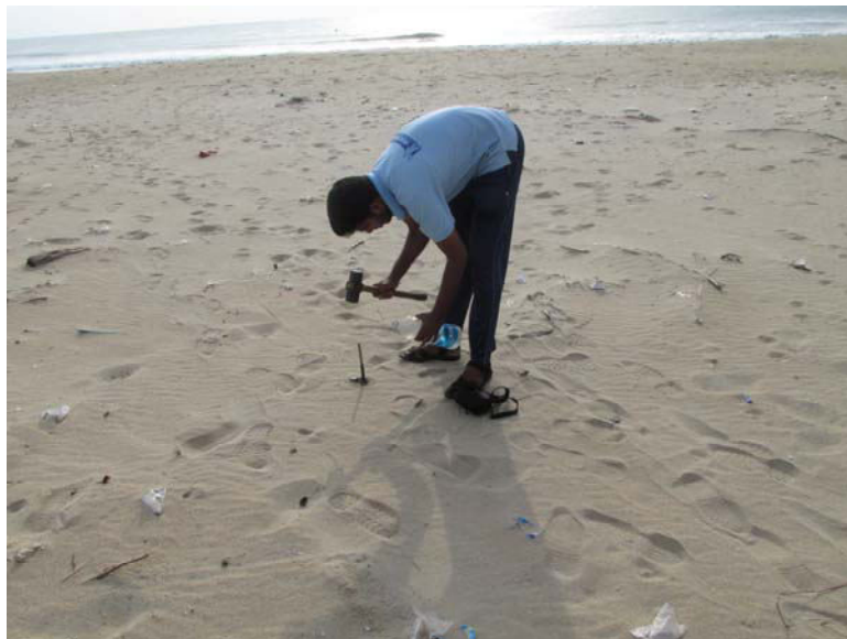
1 D sounding using Schlumberger Configuration
