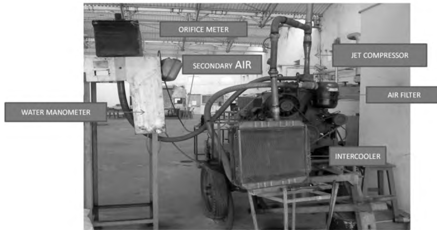
Fig.16 Experimental setup of EGR run jet compressor fitted to a diesel engine.
