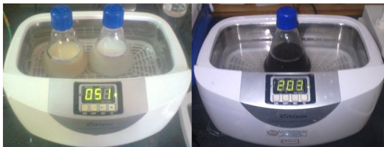
Fig.5.11. Ultrasonication process of \text{Al}_2\text{O}_3 , ZnO and CuO Nano particles
