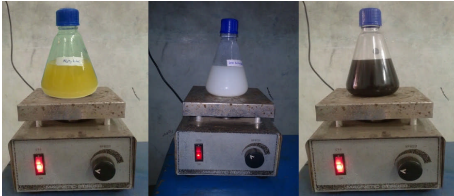
Fig.5.10. Magnetic stirring process of \text{Al}_2\text{O}_3 , ZnO and CuO nano particles
