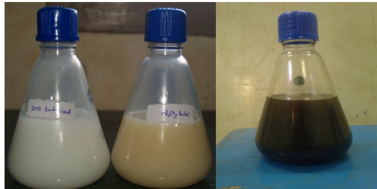
Fig.5.12. Synthesized Nano lubricants of \text{Al}_2\text{O}_3 , \text{ZnO} and \text{CuO} with no particle settlement
