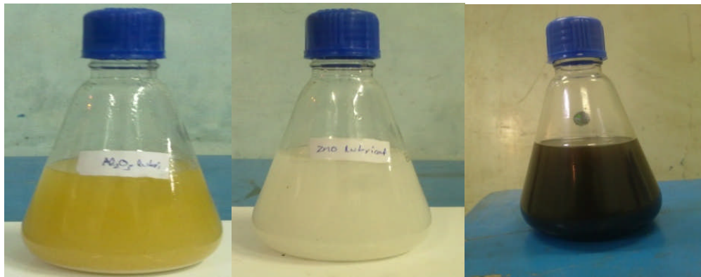
Fig.5.9. Mixing of Nano particles of Al 2 O 3 , ZnO and CuO
