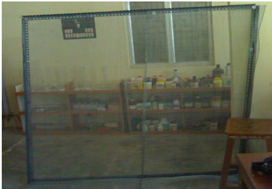
Figure 3.3 GI mesh for the drain of leachate from solid waste
