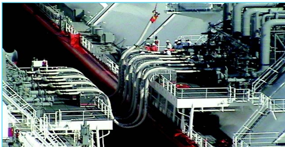
Example of unloading of LNG through Flexible Cryogenic Hoses
