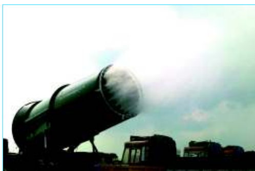
Dust Suppression Sprayer loaded on Truck
