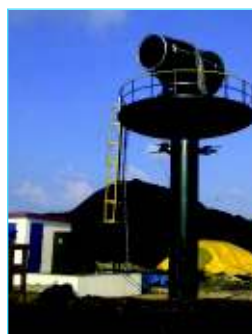
Tower Mounted Dust Suppression Sprayer
